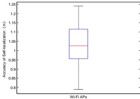
Figure 6. Detection Error of Wi-Fi APs
