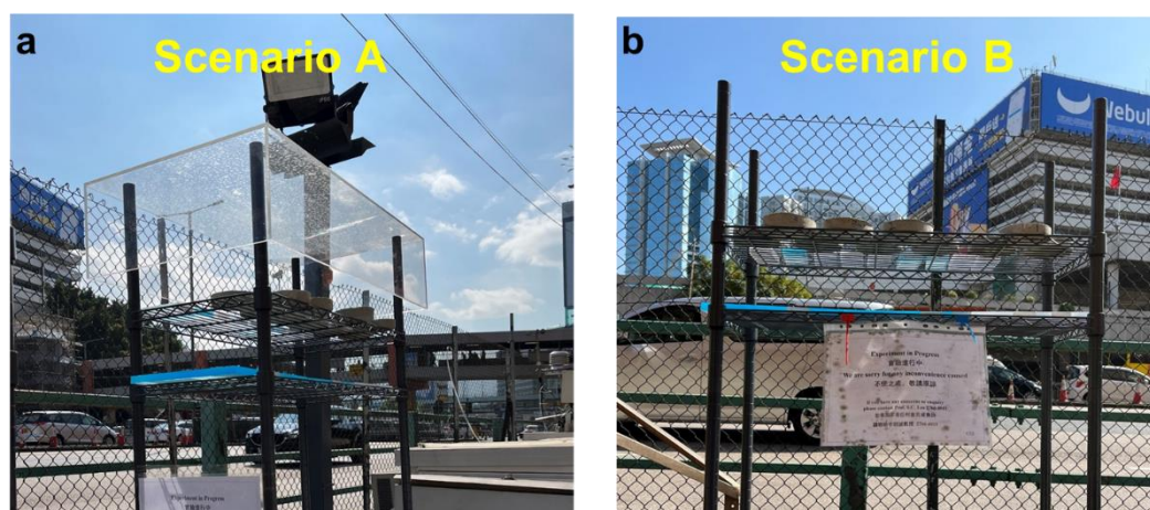
Fig. S13. Photos of set-up for Scenario A with a transparent cover (a) and Scenario B without a transparent cover (b) of field trials.
