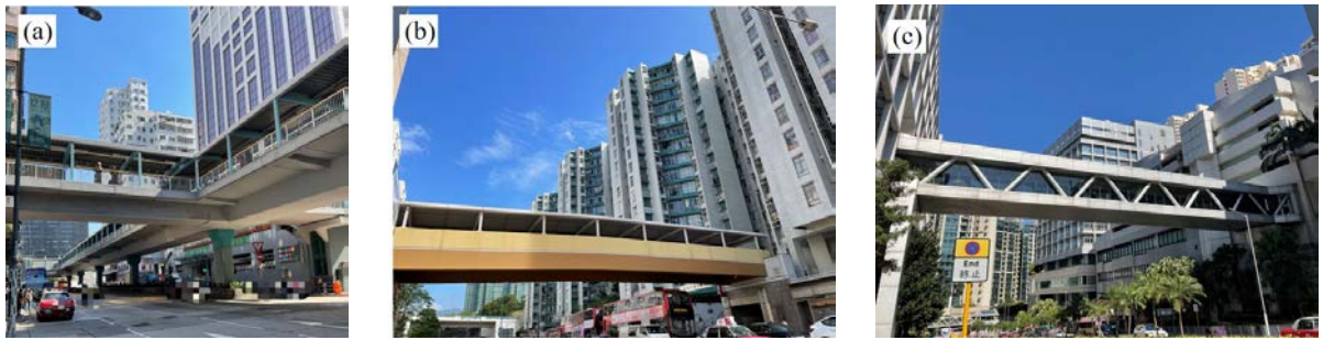
Fig. 1. Examples of elevated walkways in Hong Kong photographed by authors: (a) Type A—open/steel railing, (b) Type B—semi-hermetic/concrete, (c) Type C—hermetic/glass.
