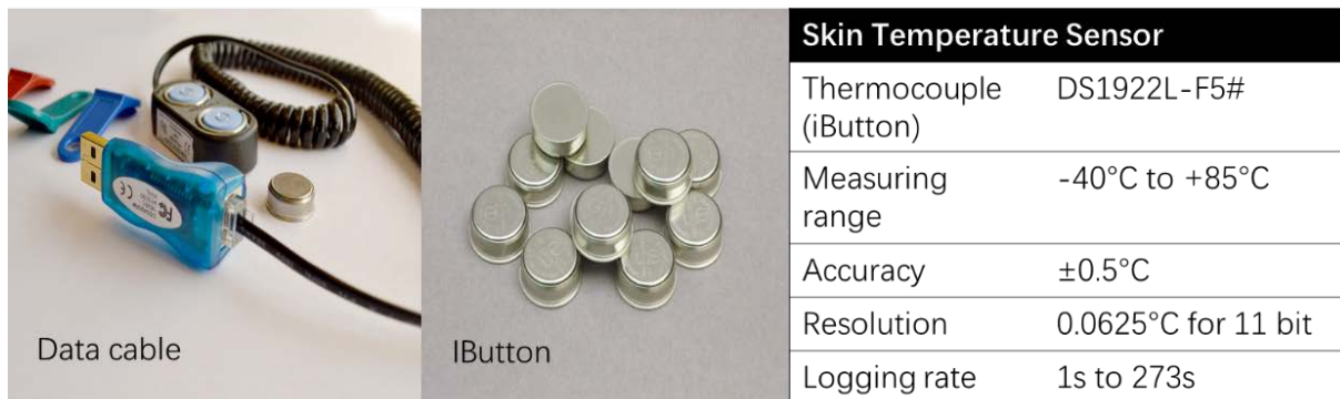
Figure 4 Thermocouples (i-Button) for measuring skin temperature.
