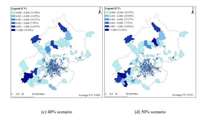
Fig. 10 Spatial distributions of Coefficient of Variation (CV) in the scenarios with different numbers of charging stations to be deployed at the TAZ level
