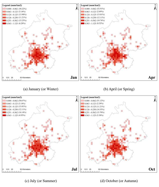
Fig. 8 Spatial distributions of charging stations to be deployed at the resolution of 4×4 km grid
