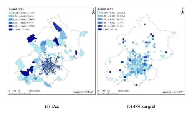
Fig. 9 Spatial distributions of Coefficient of Variation (CV) for charging stations to be deployed at different spatial resolutions in the baseline scenario
