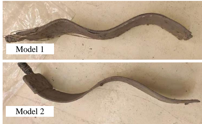
Fig. 13 Photos of the bent PVDs after tests
