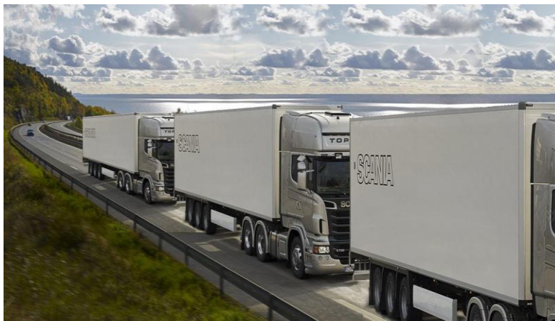
Figure 1. Illustration of a three-truck platoon (Larsson et al., 2015)
