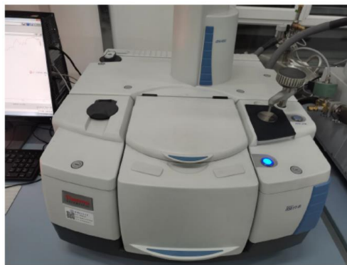
Fig. 2. The FTIR device with ATR module.
