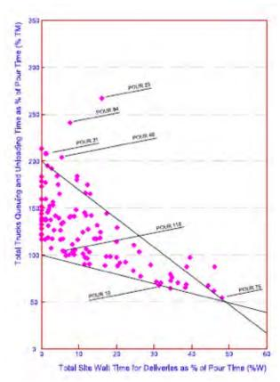
Figure 3: Matching of truckmixer queuing and unloading on site versus placing crew waiting for truckmixer deliveries (118 pours) in 1999/2000
