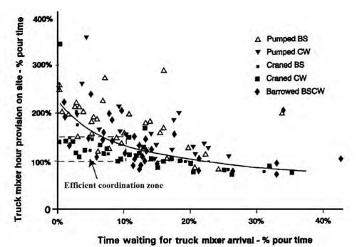
Figure 2: Truckmixer hour provision on site versus waiting for truckmixer arrival (137 pours) in 1994
