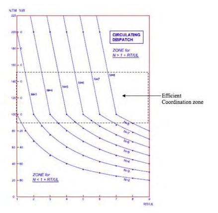
Figure 4: Circulating dispatch relationships between RT/UL, N, %W and %TM
