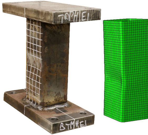
(b) Section yielding failure mode (H80×80×4-BC-e80)
