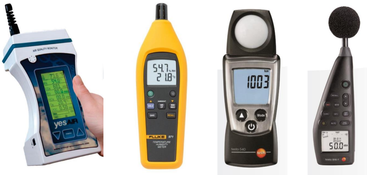
(i) Air Quality Monitoring Device (ii) Temp. & Humidity Meter (iii) Lux Meter (iv) Sound level meter (a) Tools and instruments for environmental measurements Fig. 11. Portable instruments to measure physical defects and environment
