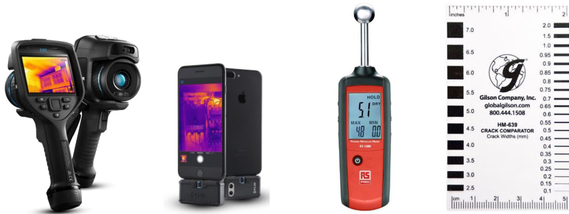
(i) Portable Infrared thermal cameras (ii) Moisture Meter (iii) Crack width Scale (a) Tools and instruments for physical defects inspection
