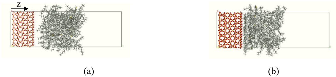
223 224 Figure 7. Initial configuration (a) and equilibrated configuration (b) of the interface model in dry 225 condition. A vacuum layer of Å was placed on top of the bitumen layer to avoid interaction across 226 the mirror image.
