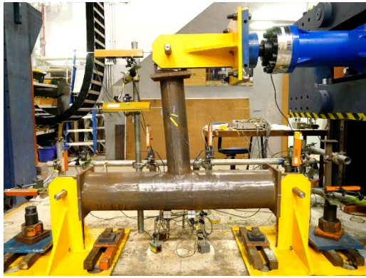
Deformed shape at the 36 th cycle \Delta_{j,x} = -52.6 \text{ mm}
