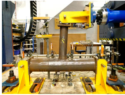
Deformed shape at the 36 th cycle \Delta_{j,x} = 59.5 \text{ mm}
