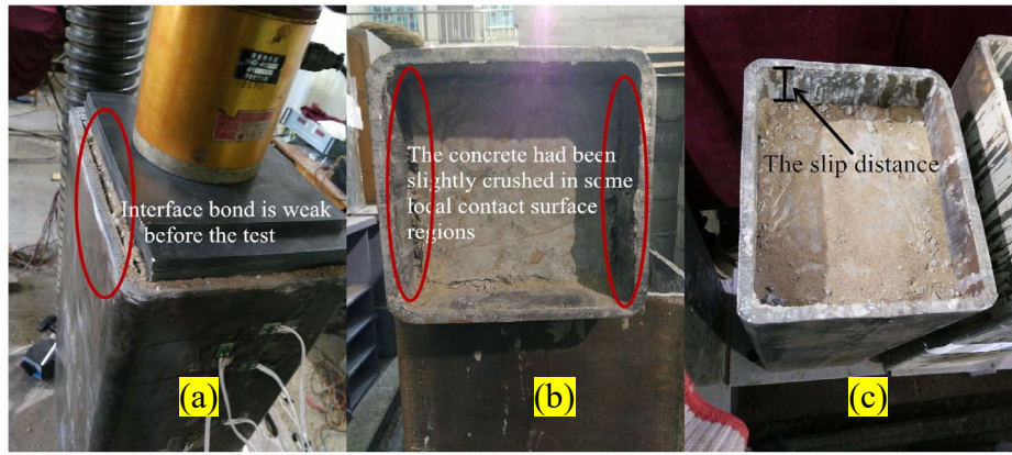
(a) Application of load (b) Concrete-steel interface (c) Slip
