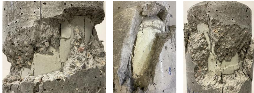
(c) Splitting of inner pultruded FRP tube
