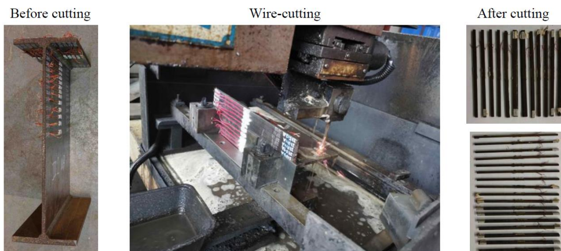
277 278 Figure 14. Sectioning of I-section test specimens for residual stress measurement
