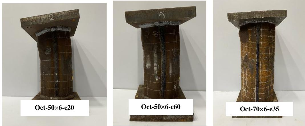
Fig. 6. Failure modes of typical test specimens.
