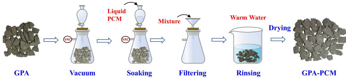
Fig. 4 Schematic illustration of the preparation process for GPA-PCM.
