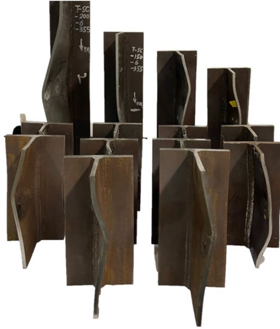
Fig. 12. Typical local buckling mode of representative specimens.
