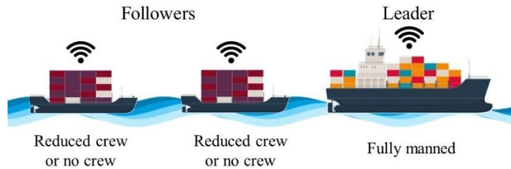
Fig. 1. The vessel train concept of NOVIMAR.
