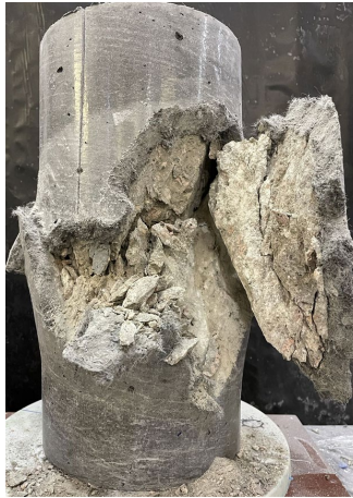
Fig. 17 Crushing of HSC core
