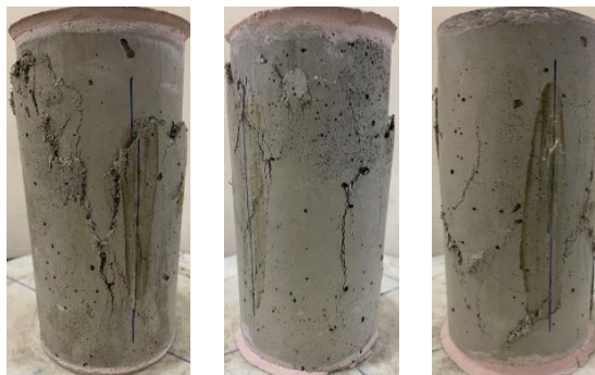
(a) Failure of plain ECC cylinder
