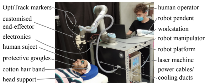
Fig. 15. The detailed illustration of the proposed robotic prototype and its components.
