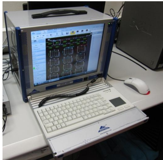
Figure S11. Data acquisition equipment for in-situ ballistic impact measurement.
