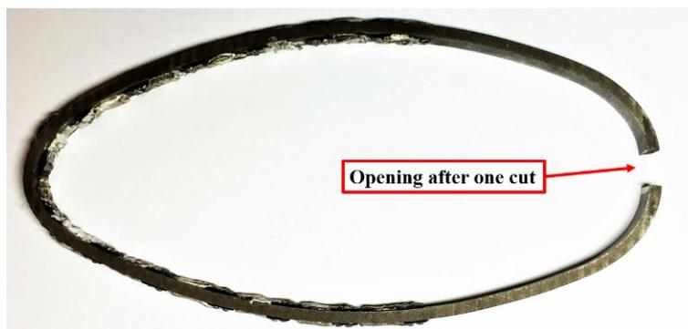
Figure 11. Deformed transverse ring of EHS 150×70×3 after cutting
