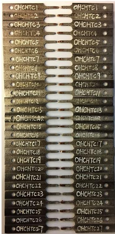
Figure 5. Failed coupon specimens extracted from the half-section of EHS 150×70×3
