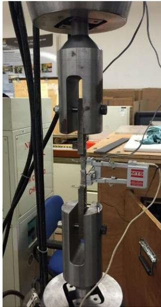
Figure 2. Setup of coupon tests of EHS
