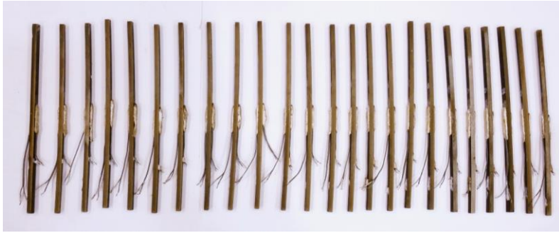
d) Deformed steel strips cut from Section C1-nw
