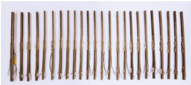
e) Deformed steel strips cut from Section C1
