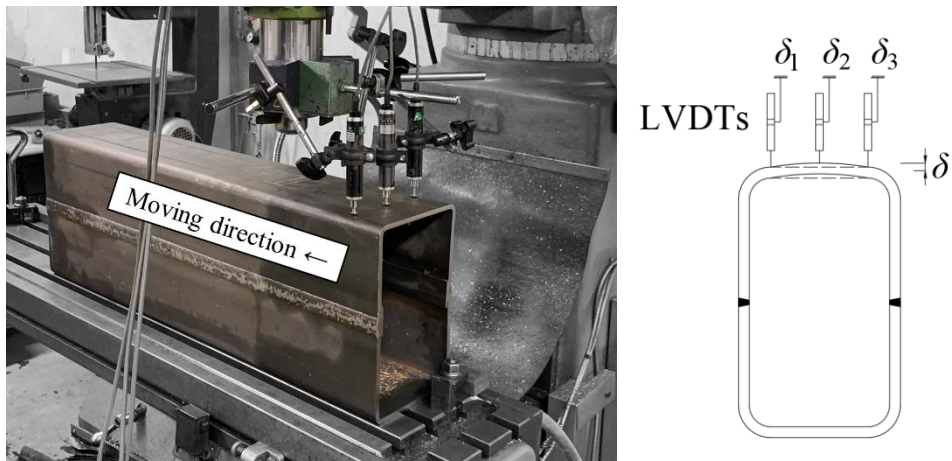
Fig. 8. Instrumentation of the local imperfection measurement.
