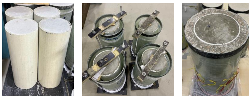
181 182 Fig. 7 Preparation process of GFRP-concrete double tube composite columns 183
