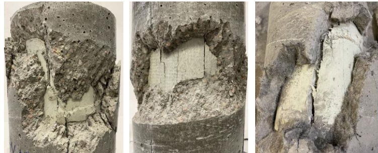
(c) Splitting failure of inner pultruded GFRP tube
