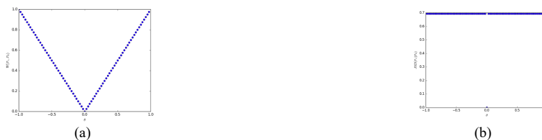
Figure 17. \rho(P_\theta, P_0) as a function of \theta , (a) \rho is the EM distance (b) \rho is the JSD. The EM plot is continuous and gives a usable gradient everywhere, whereas JS plot is not continuous and does not give a usable gradient. Figure from [35].
