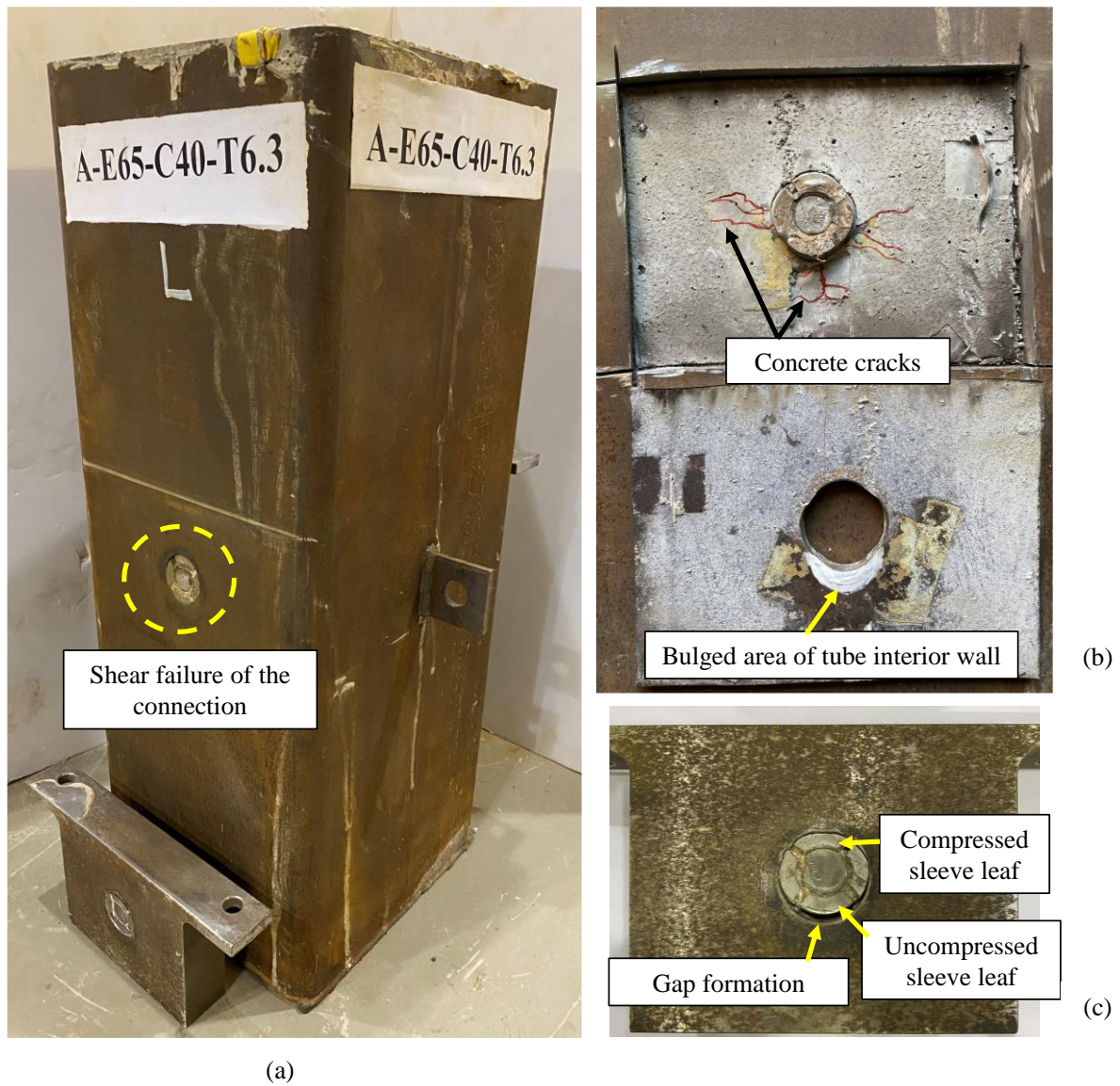
Fig. 15: (a) Specimen A-E65-C40-T6.3 after connection failure; (b) Damages in concrete and tube wall; (c) Fractured bolt after test.
