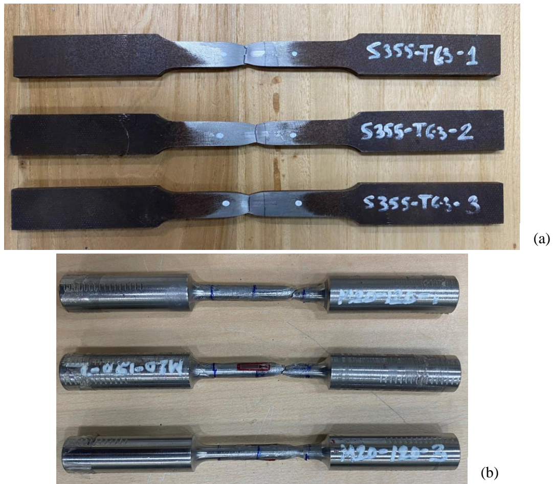
Fig. 9: Tested (a) tube flat coupons; (b) bolt coupons.
