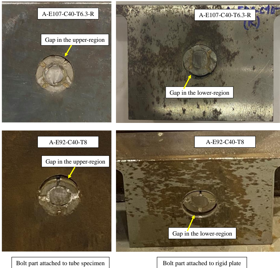
Fig. 18: Positioning of bolt after shear failure of connection.
