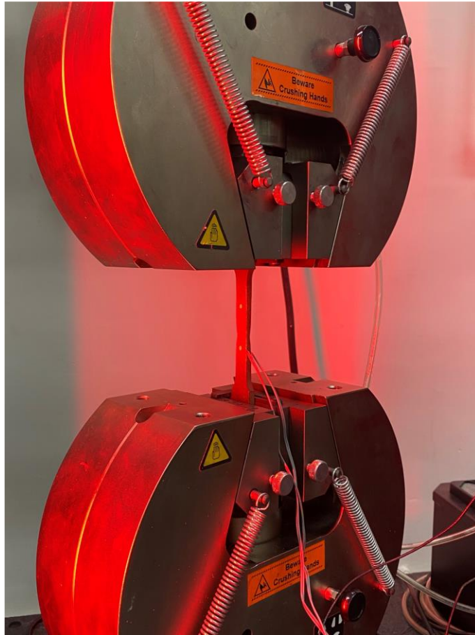
Fig. 8: Tensile testing system for steel tube coupons using Instron UTM.
