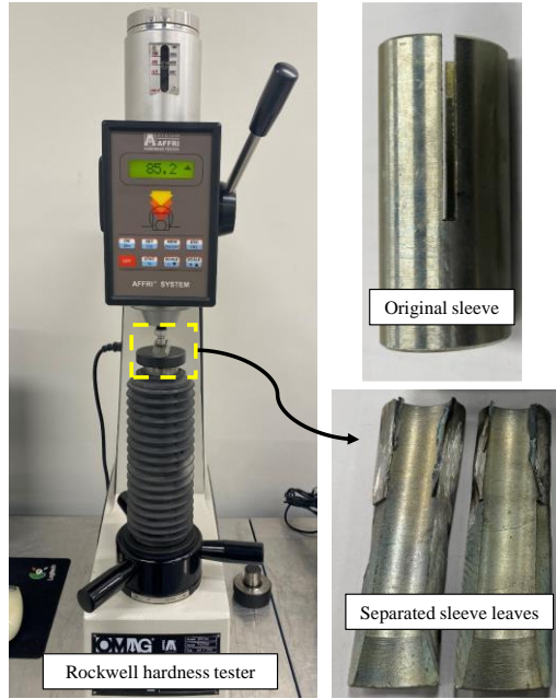
Fig.8: Hardness measurement for bolt sleeve component.
