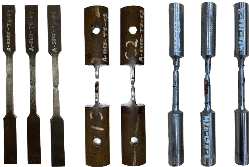
(a) Steel flat coupons
