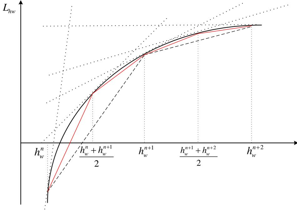
Fig. C1. The illustration of breakpoints updating
