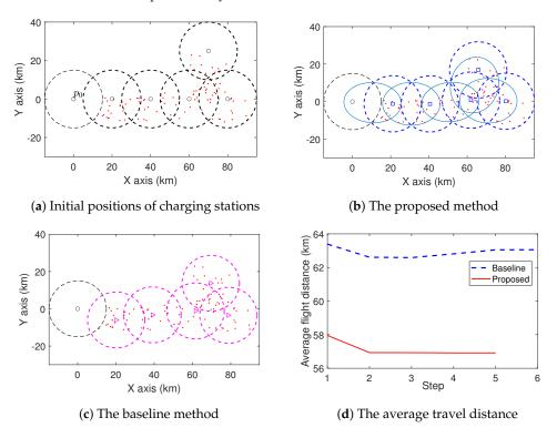
**Figure 8.** Comparison of the proposed method and baseline method in the case with five charging stations. The sites are represented by red dots.
