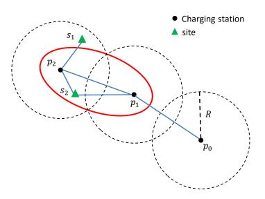
**Figure 2.** Illustrative example of the connections between site nodes and charging station nodes. Although both  $s_1$  and  $s_2$  are located within the circle centred at  $p_2$ ,  $s_1$  connects with  $p_2$  but not  $p_1$ , while  $s_2$  connects with both  $p_1$  and  $p_2$ . This is because  $|p_1, s_1| + |s_1, p_2| > 2R$ , while  $|p_1, s_2| + |s_2, p_2| \le 2R$ .
