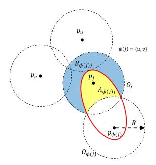
**Figure 4.** Illustration of the coverage of a pair of child-parent charging stations  $p_j$  and  $p_{\phi(j)}$ . Vertex  $\phi(j)$  is the parent of vertex j, and the set of the child vertices of Vertex j consists of u and v, i.e.,  $\psi(j) = \{u, v\}$ .
