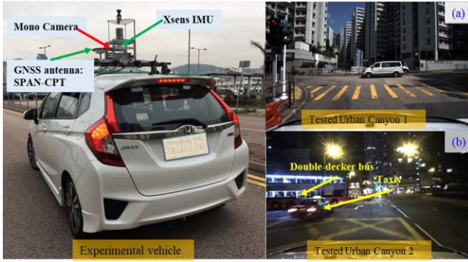
Fig. 6. Experimental setup and the evaluated scenes (a) and (b).
