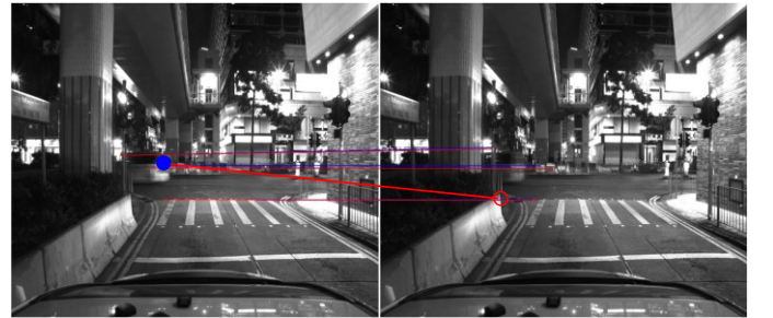
Fig. 1. Example of a failure of feature tracking of optical flow.
