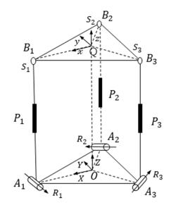
Figure 9. The 3-SPR kinematics model.
