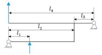
Figure 4. Schematic diagram of the lever amplification mechanism.
