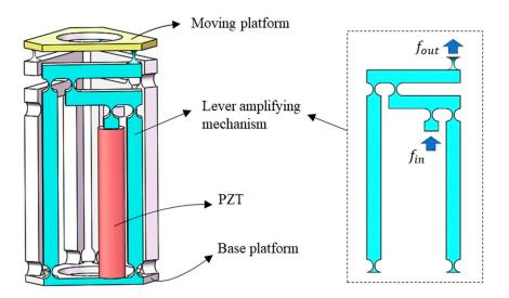
Figure 3. Model of a 3-DOF flexible micro-motion platform.
