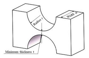
Figure 2. Straight round flexure hinge.
