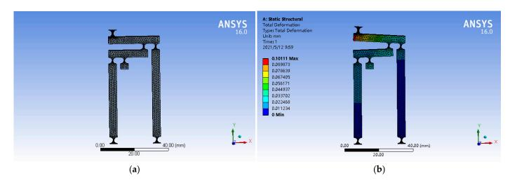
Figure 5. Meshing results of the mechanism (a); simulation of amplifier mechanism (b).
