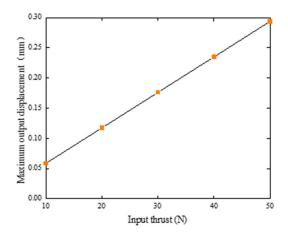
Figure 7. Relationship input thrust and maximum output displacement.
