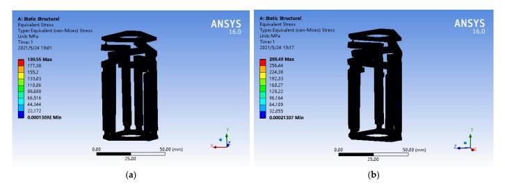
**Figure 8.** Static simulation of maximum stress value. (a) Three branches chain loaded displacement of 30  $\mu$ m; (b) three branches chain loaded thrust of 50 N.
