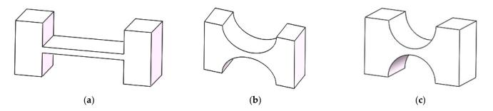
Figure 1. Different notched flexure hinges: (a) right-angle incision; (b) elliptical incision; (c) circular incision.
