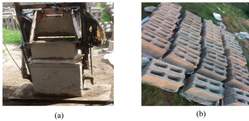
Figure 7. (a) Automated hollow block vibrated compaction (b) Hollow block placement on wooden pallette for curing in natural air and sunlight.
