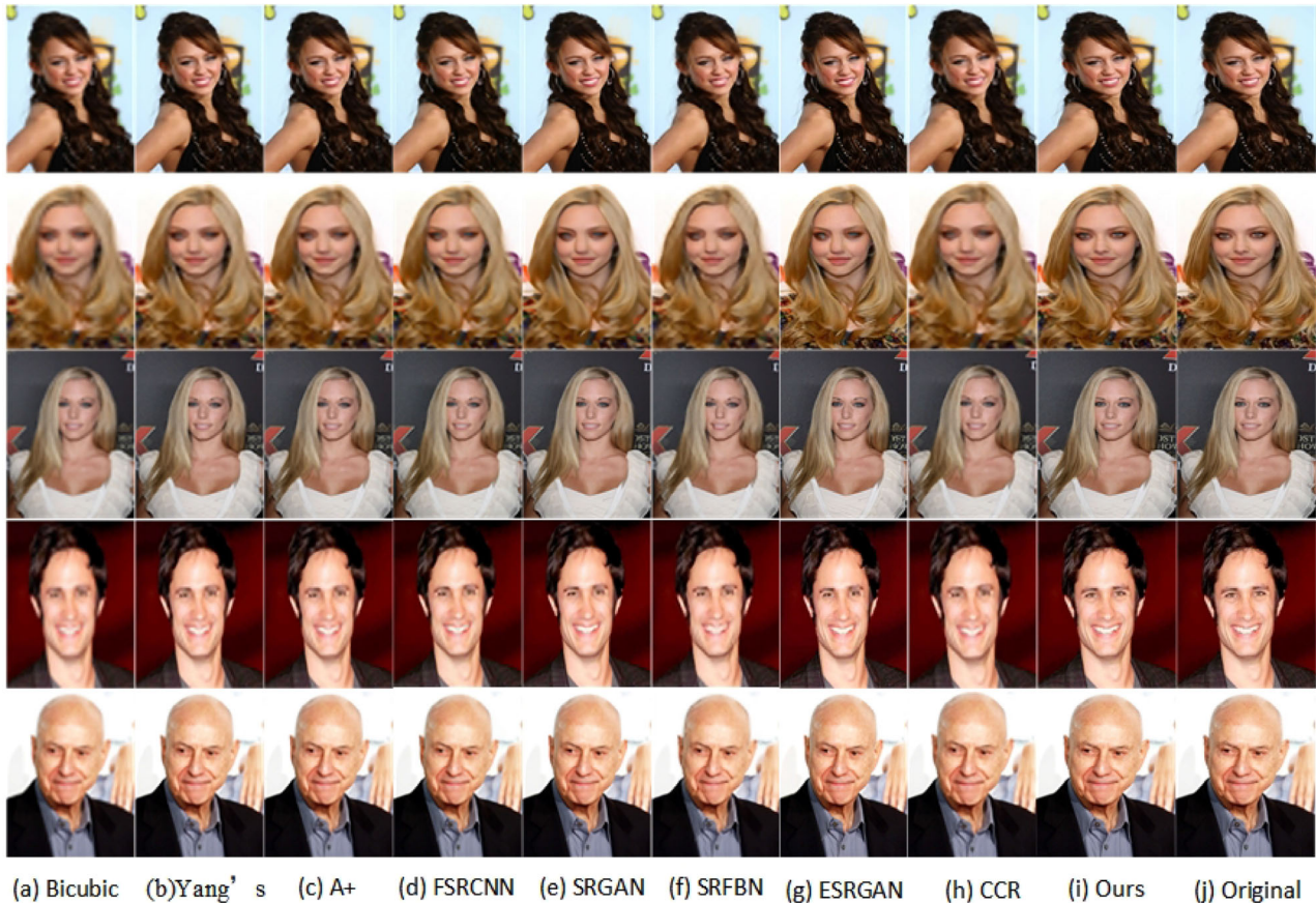
FIGURE 6 Face hallucination results on the LFPW dataset for scale 4 with different methods: (a) Bicubic interpolation, (b) Yang's method, (c) A+, (d) FSRCNN, (e) SRGAN, (f) SRFBN, (g) ESRGAN, (h) CCR, (i) our method and (j) the original HR faces
