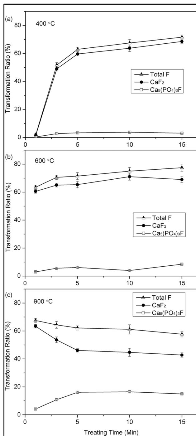
Fig. 6. Effect of thermal treatment time on the fluorine transformation efficiencies. The transformation ratio (TR) values for the sludge + PFOS +  $\text{Ca}(\text{OH})_2$  samples (Ca/F molar ratio of 2:1) were obtained by heating samples at 400 °C, 600 °C, and 900 °C with different retention times (Wang et al., 2013).
