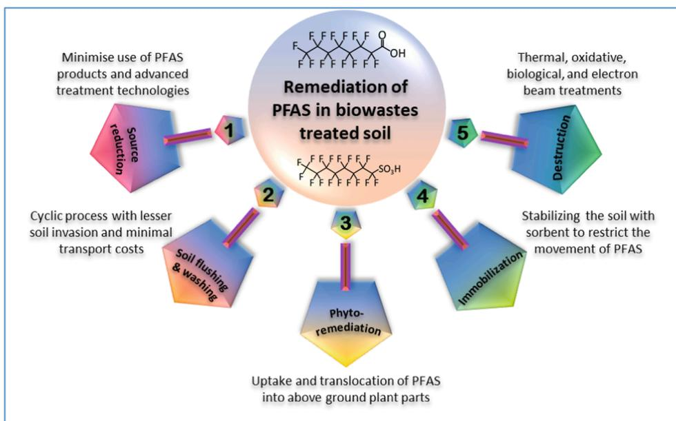
Fig. 4. Remediation options for PFAS in biowastes and soils treated with biowastes.
