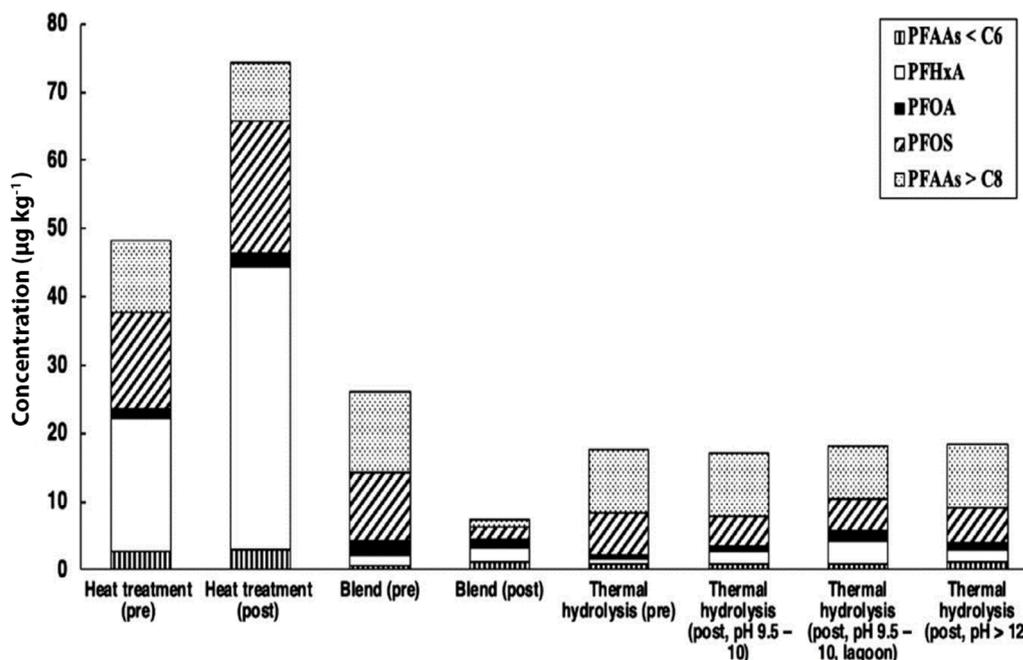
Fig. 5. PFAA loads ( $\mu\text{g kg}^{-1}$ , dw) for the < 2 mm particle size fraction of the samples. Pre: before post-treatment process (the Class A or B biosolids) and post: after post-treatment process. PFAAs < C6 include PFBA and PFBS, and PFAAs > C8 include PFNA, PFDA, PFUDA, PFDOA, PFTDA, and PFTeDA. (Lazcano et al., 2019).
