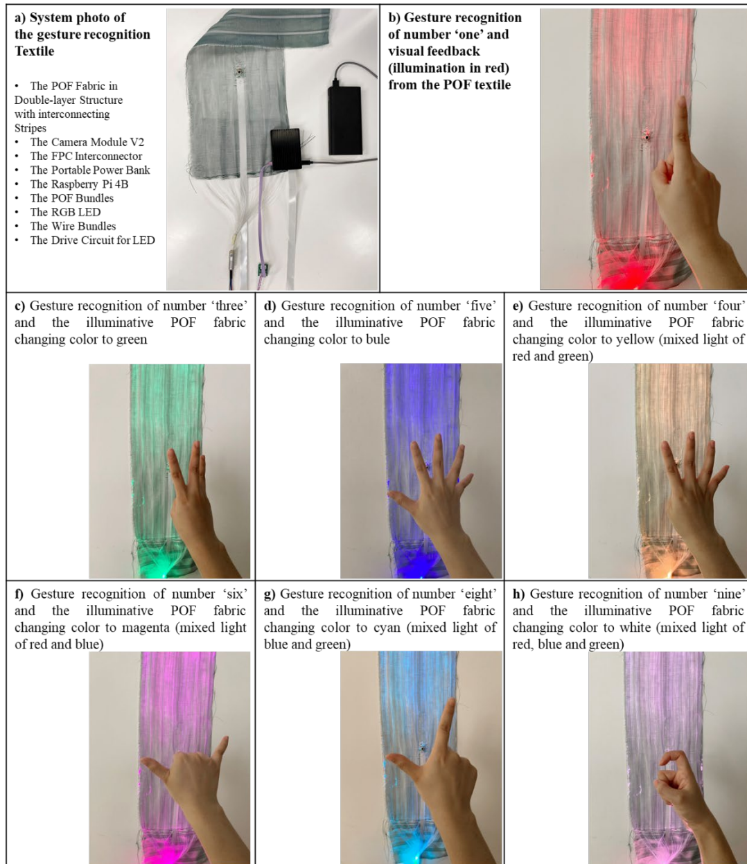
Figure 7a) shows the system of the gesture recognition textile with all components in situ; b) illustrates gesture recognition of number 'one' with visual feedback (illumination in red) from the POF textile; photographs c)-h) relate to gesture recognition of numbers 'three, five, four, six, eight, nine', with the illuminative POF fabric correspondingly changing colour to green, blue, yellow, magenta, cyan and white.
