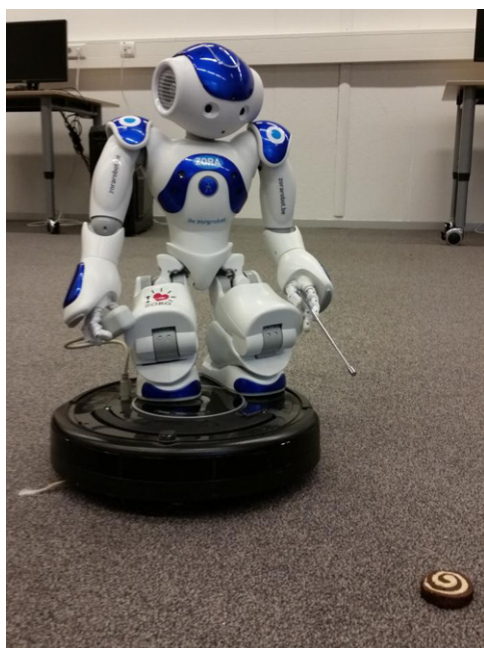
Fig. 1. Nao robot with Zora software mounted on a Roomba vacuum cleaner.
