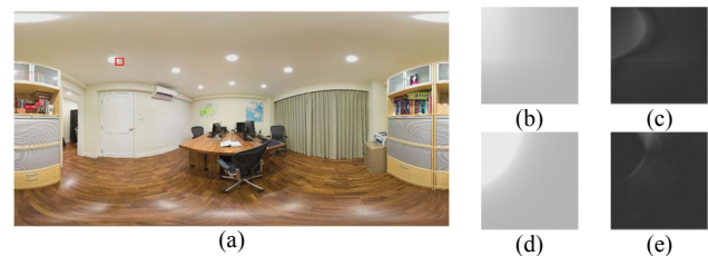
Fig. 2. (a) An example of ERP image, (b)-(c) the prediction and the corresponding residue (lighter color means larger difference) of the conventional intra mode, (d)-(e) the prediction and the corresponding residue (contrast-enhanced) of our proposed 360-degree intra mode.
