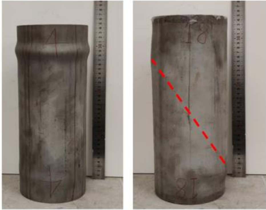
Figure 10: Failure modes of 139.4×3.0 ( left ) and 139.4×3.0-SW-C70 ( right ).
