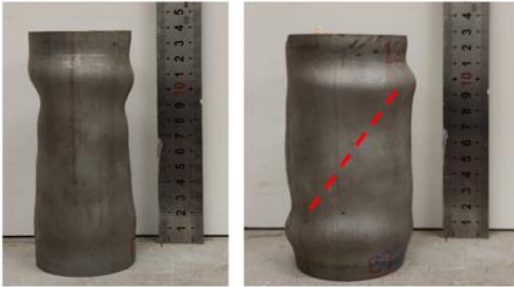
Figure 8: Failure modes of 60.5×2.8 ( left ) and 60.5×2.8-SW-C70 ( right ).
