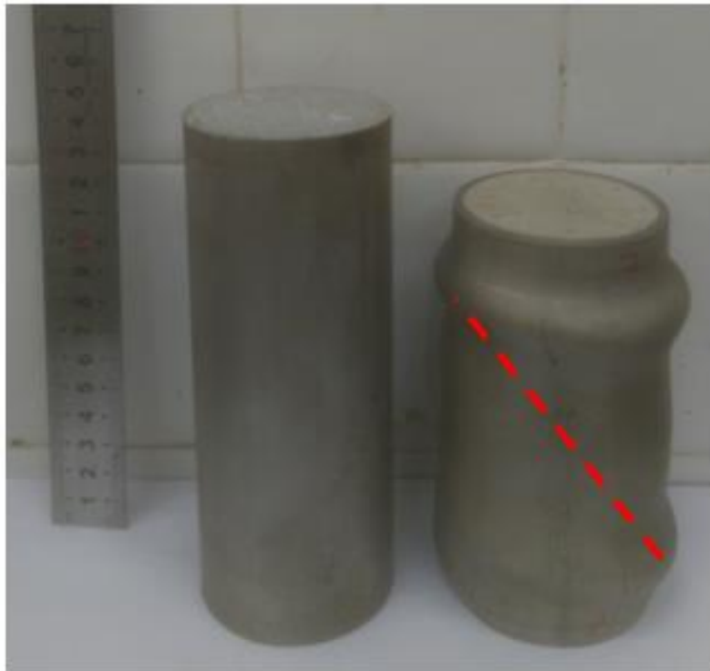
Figure 12: Length and shape of 60.5×2.8-SW-C35 before testing ( left ) and after testing ( right ).
