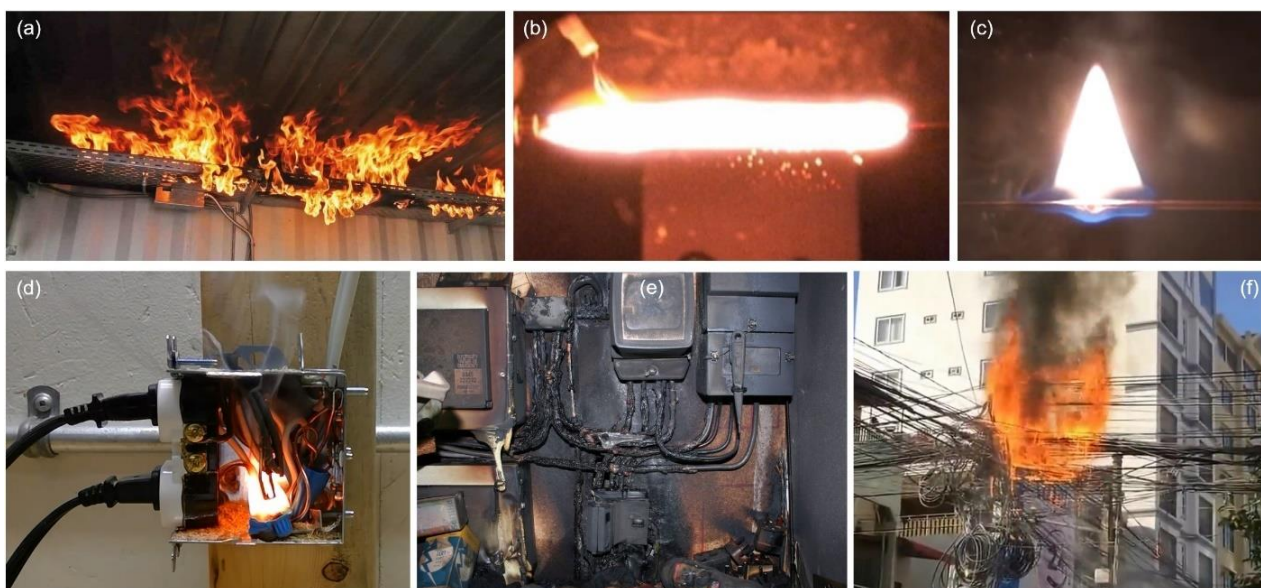
Figure 1. Typical wire fire accidents (a) in a ceiling wire tray [59], (b) overload ignition in microgravity [18], (c) flame spread over a thin laboratory wire [60], (d) fire starts at the wiring connection [61], (e) fire damage caused by loose wiring connection [62], and (f) in tangled wires above the street [63].
