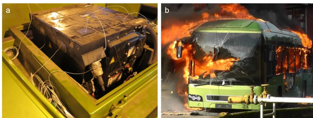
Figure 21. A full-scale fire test of the electric-diesel hybrid bus (a) battery pack with thermocouples, and (b) bus in fire at 32.5 min [153].
