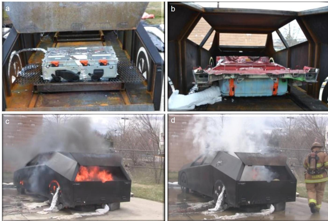
Figure 22. Full-scale fire-suppression test of EV battery packs inside a vehicle model: (a) Type A battery pack; (b) Type B battery pack with interior components; (c) fire behaviours of Battery A; and (d) fire suppression efforts [65,73].
