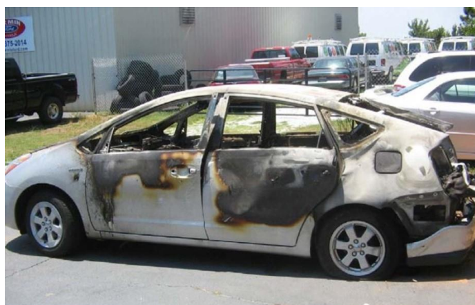
Figure 14. A Toyota Prius converted to a plug-in hybrid electric vehicle by the owner and was damaged by the battery fire. This fire accident resulted from the thermal runaway of the battery [122].
