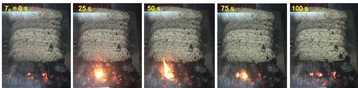
Fig. 9. Un-sustained smoldering-to-flaming transition under the wind velocity of 2.8 m/s.
