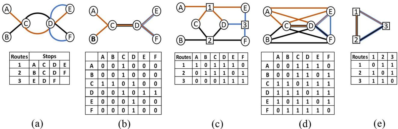
Fig. 1: (a) Simple public transport map with stations A–F being serviced by route no. 1 (shaded orange), no. 2 (black), and no. 3 (blue); (b) L-space graph; (c) B-space bipartite graph (route nodes are shown as squares); (d) P-space graph (complete sub-graph corresponding to route no. 1 is highlighted in orange); (e) C-space graph of routes. The matrix of connectivity is shown below the corresponding network representation.
