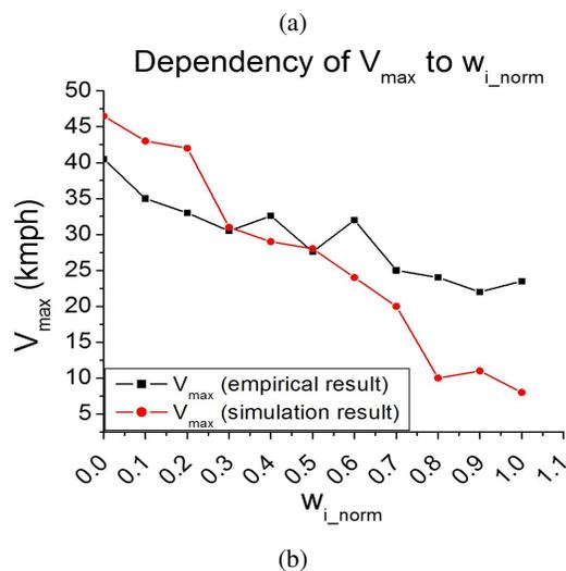
Fig. 8: (a) Snapshot of the SUMO simulator; and (b) comparison of the simulation and empirical results for the dependency of vehicular speed on node weight.
