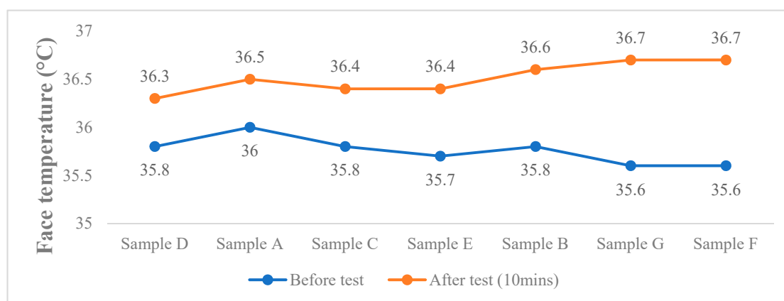
Figure 5. Recorded face temperature difference, in-mask temperature and in-mask humidity of different masks in the wear trial. Note: In-mask temp. (°C): Simple D = 32.5; Simple A = 34.2; Simple C = 33.1; Simple E = 34.5; Sample B = 34.1; Sample G = 34; Sample F = 34.2. In-mask humidity (%): Simple D = 85.5; Simple A = 87; Simple C = 86; Simple E = 86.5; Sample B = 87.5; Sample G = 84.5; Sample F = 87.
