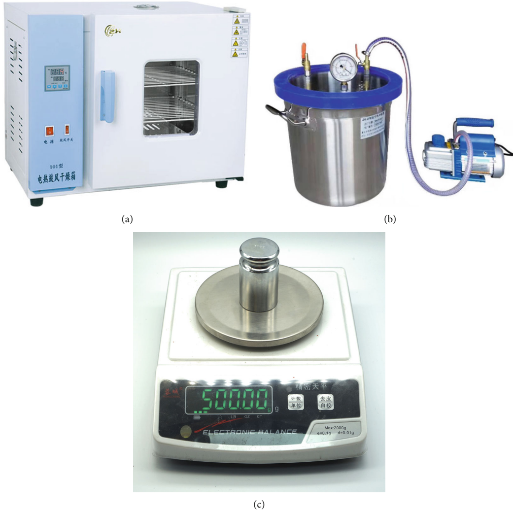
FIGURE 7: (a) Drying oven, (b) vacuum saturation device, and (c) electronic scale.
