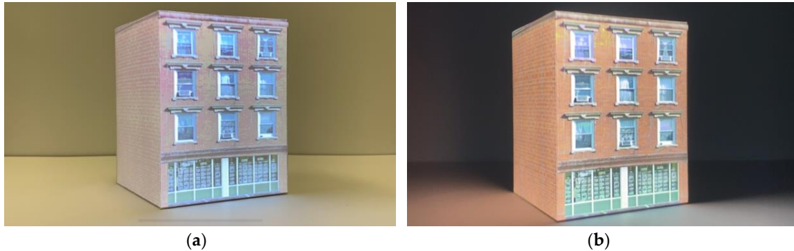
Figure 5. Comparison of projection results with illumination condition. (a) Projection with environmental electric light; (b) Projection without environmental light.
