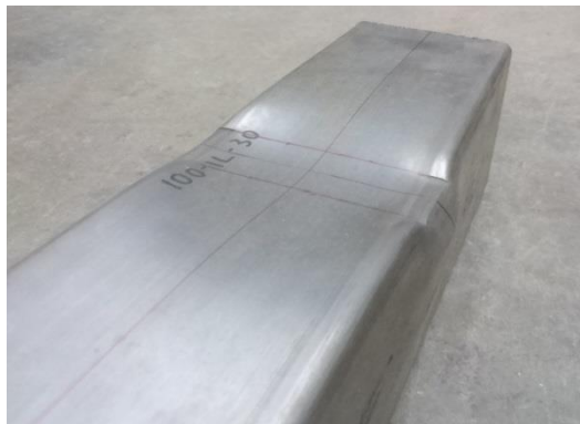
Fig. 5. Web crippling failure of specimens subjected different concentrated interior bearing loads (c) Specimen IL100×100×3.0N30
