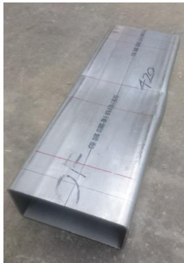
Fig. 5. Web crippling failure of specimens subjected different concentrated interior bearing loads (a) Specimen IOF80×150×3.0N60
