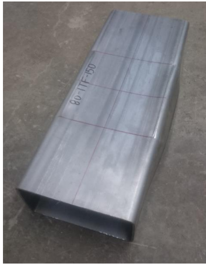
Fig. 5. Web crippling failure of specimens subjected different concentrated interior bearing loads (b) Specimen ITF80×150×3.0N150
