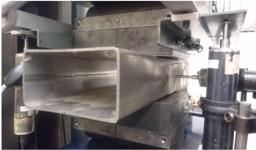
Fig. 3. Test setup specimens subjected different concentrated interior bearing loads (b) Specimen ITF80×150×3.0N150
